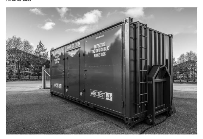
Having climate testing equipment built into a container is the optimal solution when either there is no space indoors or when other reasons require tests to be done in places where there is no real estate to place the test equipment inside.
